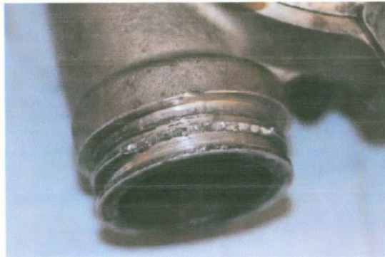
Fig. 12: Broken strip on the turbo
