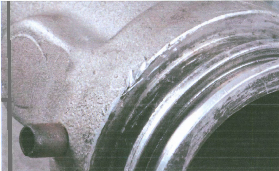
Fig. 20: Damages on the joint surface of clamp and housing which can result by e.g. leverage force using a screwdriver
