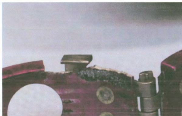
Fig. 17: Broken strip on the Wiggins clamp
