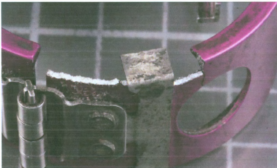
Fig. 26: Chipped edge on the clamp.
