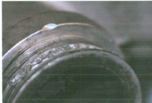
Fig. 13: Traces of leverage directly above the broken strip (e.g. with a screw driver)
