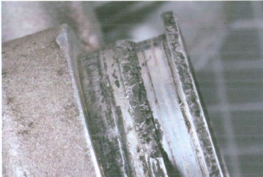
Fig. 21: Fracture surface on the turbo.
