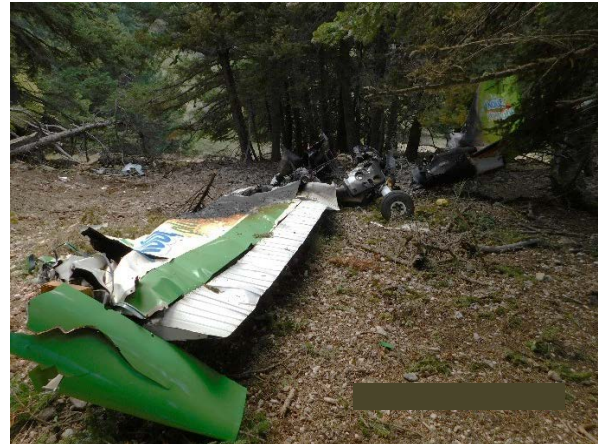
Fig. 5 The deformed airplane's left wing tip
