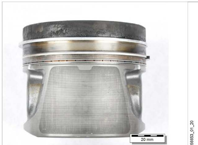
Fig. 5: Overview of the piston, skirt
