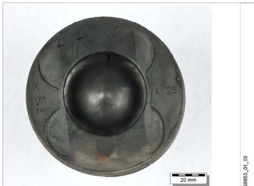
Fig. 2: Overview of the piston, top face (crown)
