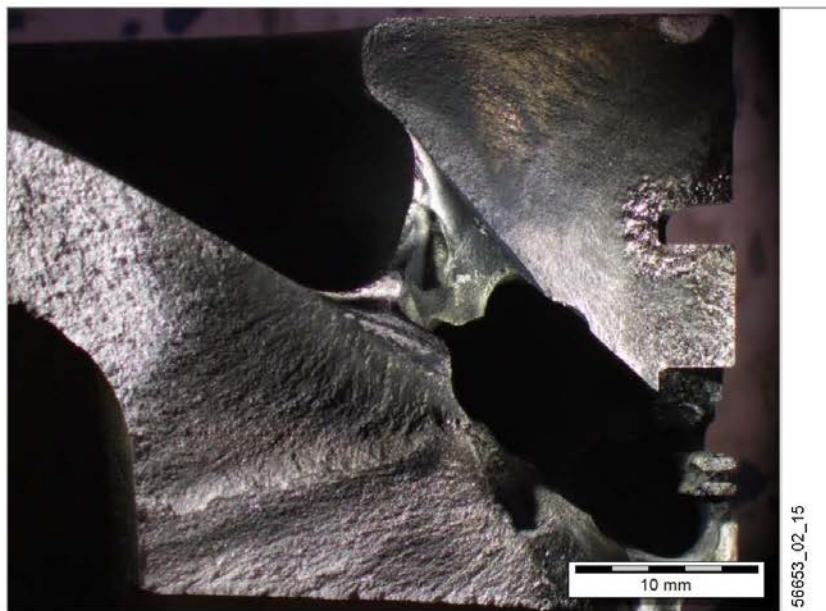
Fig. 21: Overview of the fracture surface (counter surface to fig.15)
