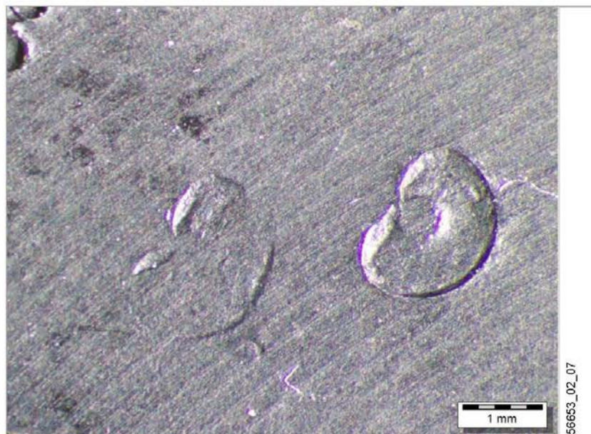
Fig. 30: Imprints of a foreign particle in the piston crown next to labelling (see also fig. 7)
