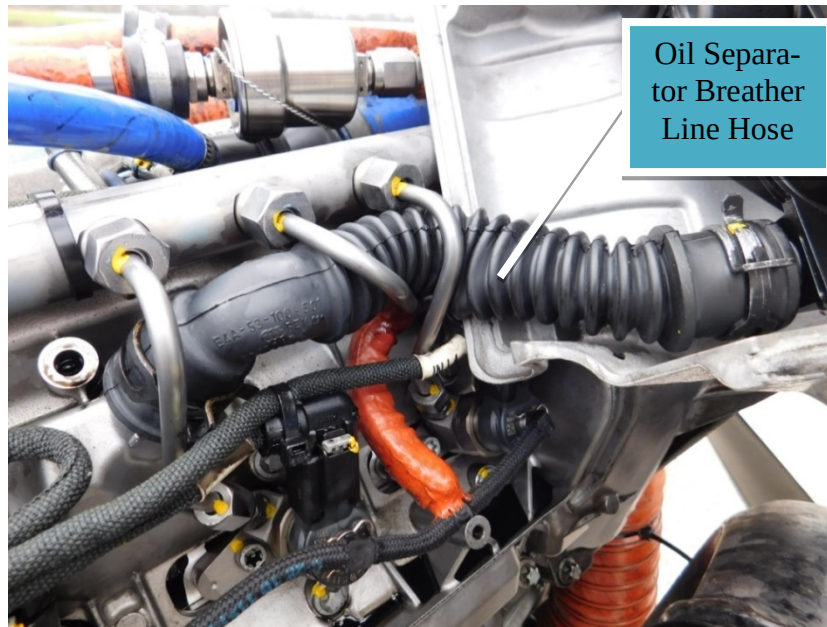
Photo 1: The oil separator breather line hose
