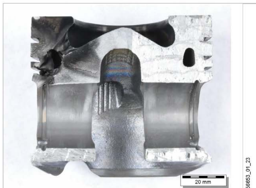
Fig. 14: Overview on the opened crack (counter surface to fig. 13)
