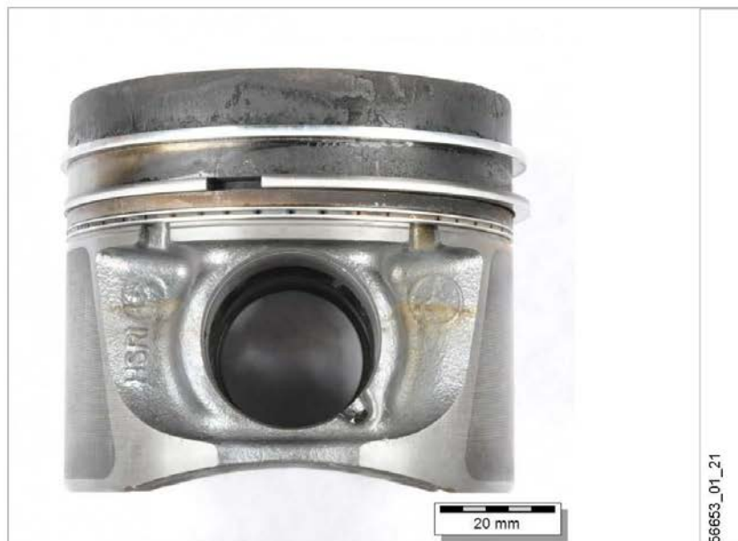
Fig. 6: Overview of the piston, side view
