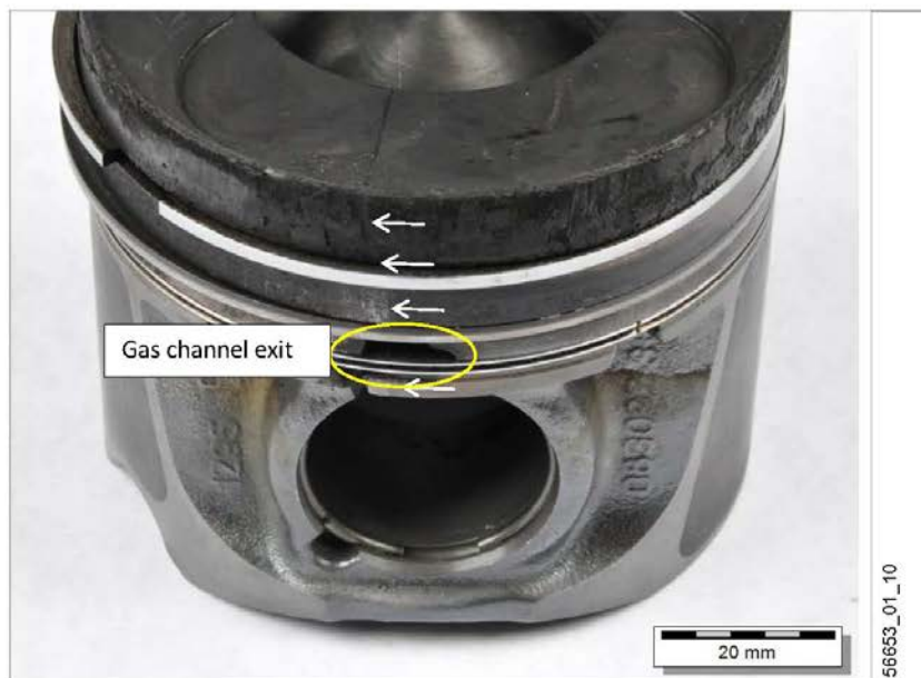
Fig. 11: Following the crack at the outer contour until it meets the piston pin bore
