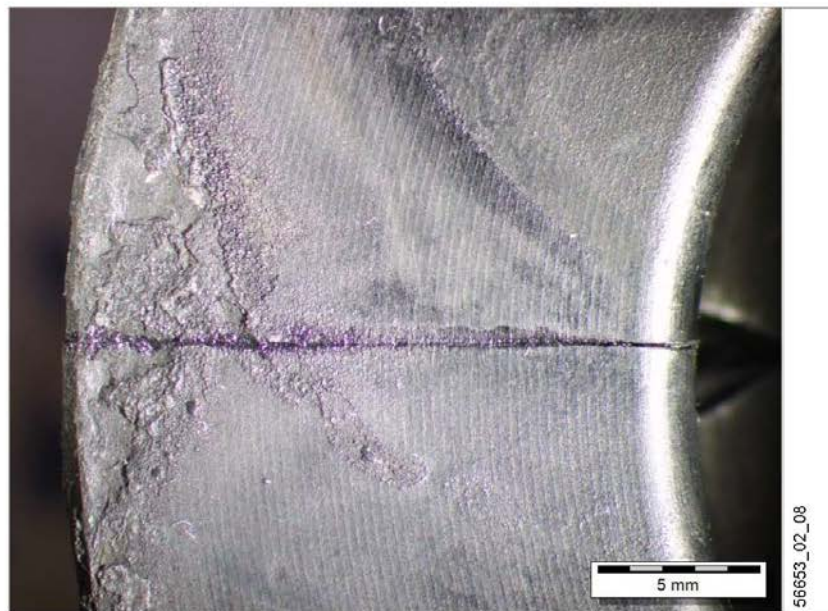
Fig. 9: Overview of the crack in the piston crown; no imprints correlate with the crack
