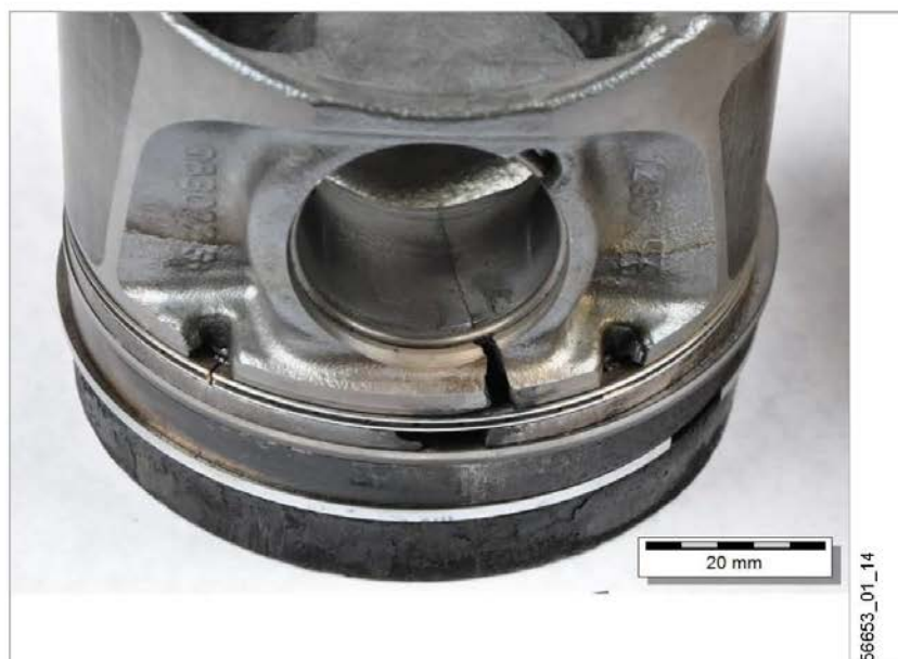
Fig. 12: The crack follows the piston pin bore until the centre area (central cone)
