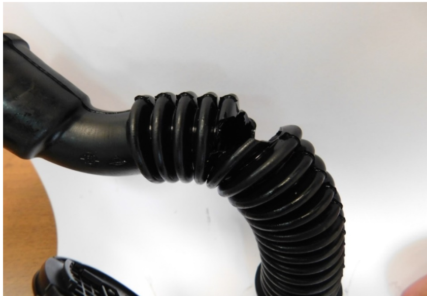
Photo 2: The torn hose of the oil separator breather line after its removal from the engine
