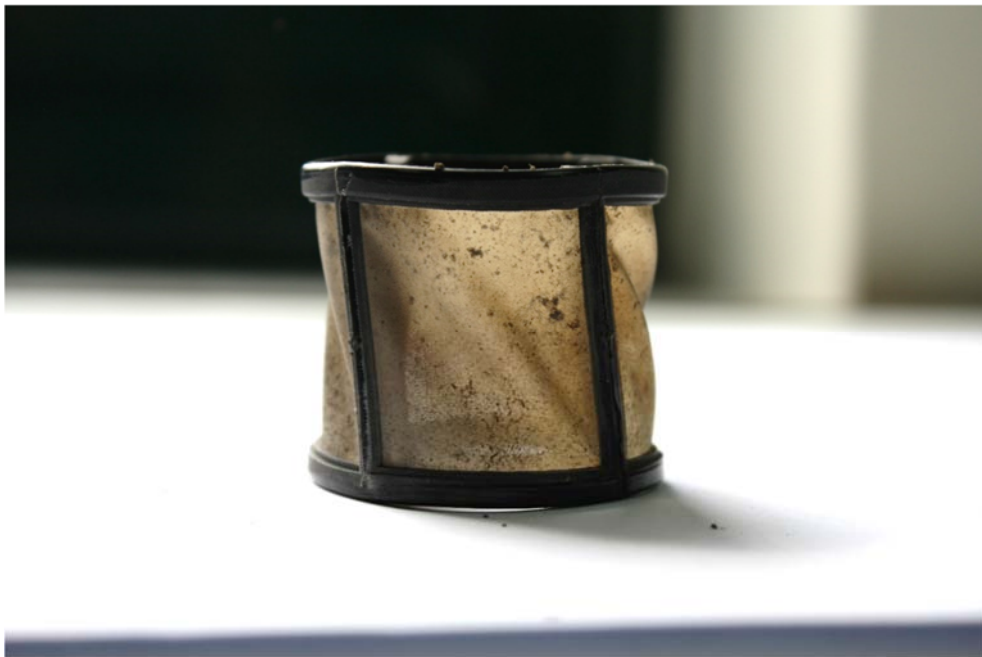
Photo 33: The filter of the electric fuel pump in the macroscopic examining it with its slight deposits.
