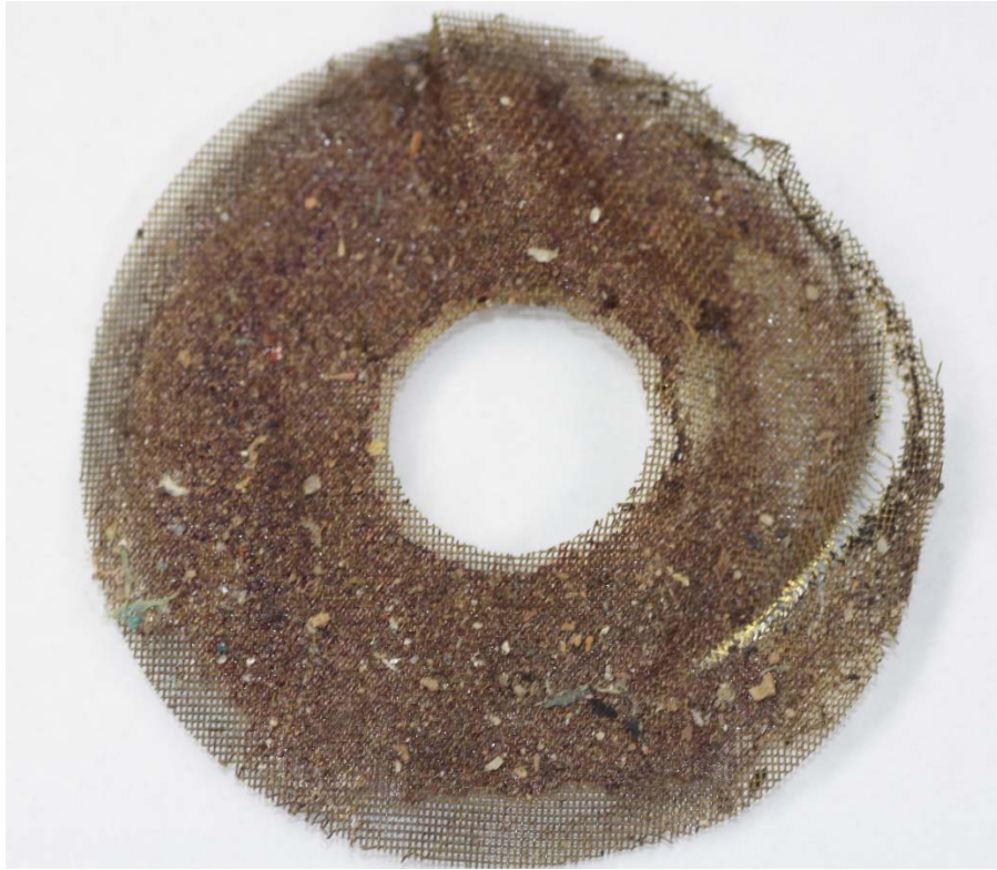
Photo 38: The inside view of the fuel filter
