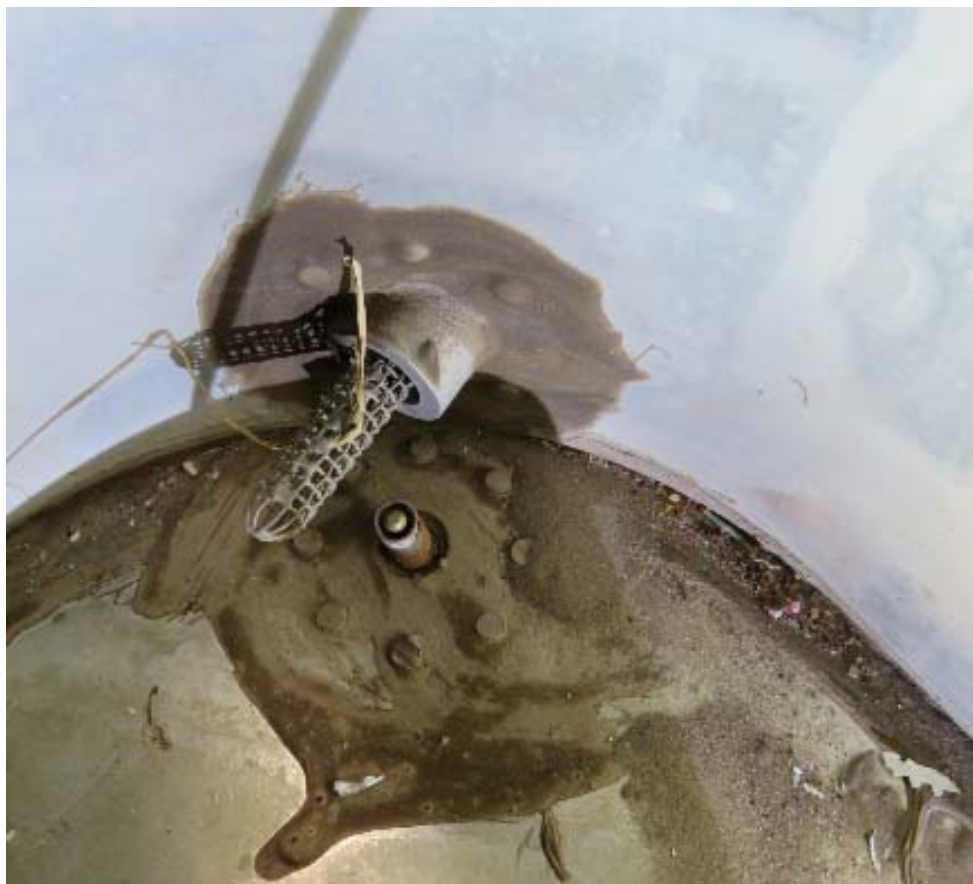
Photo 37: Sample of deposits in the left fuel tank
