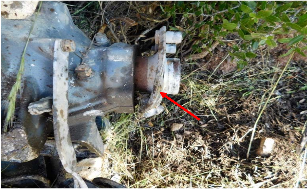
Photo 16 : The deformation of the engine shaft at the point of connection with the propeller.
