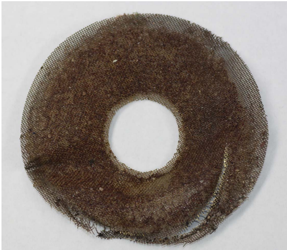
Photo 39: The outside view of the fuel filter .
