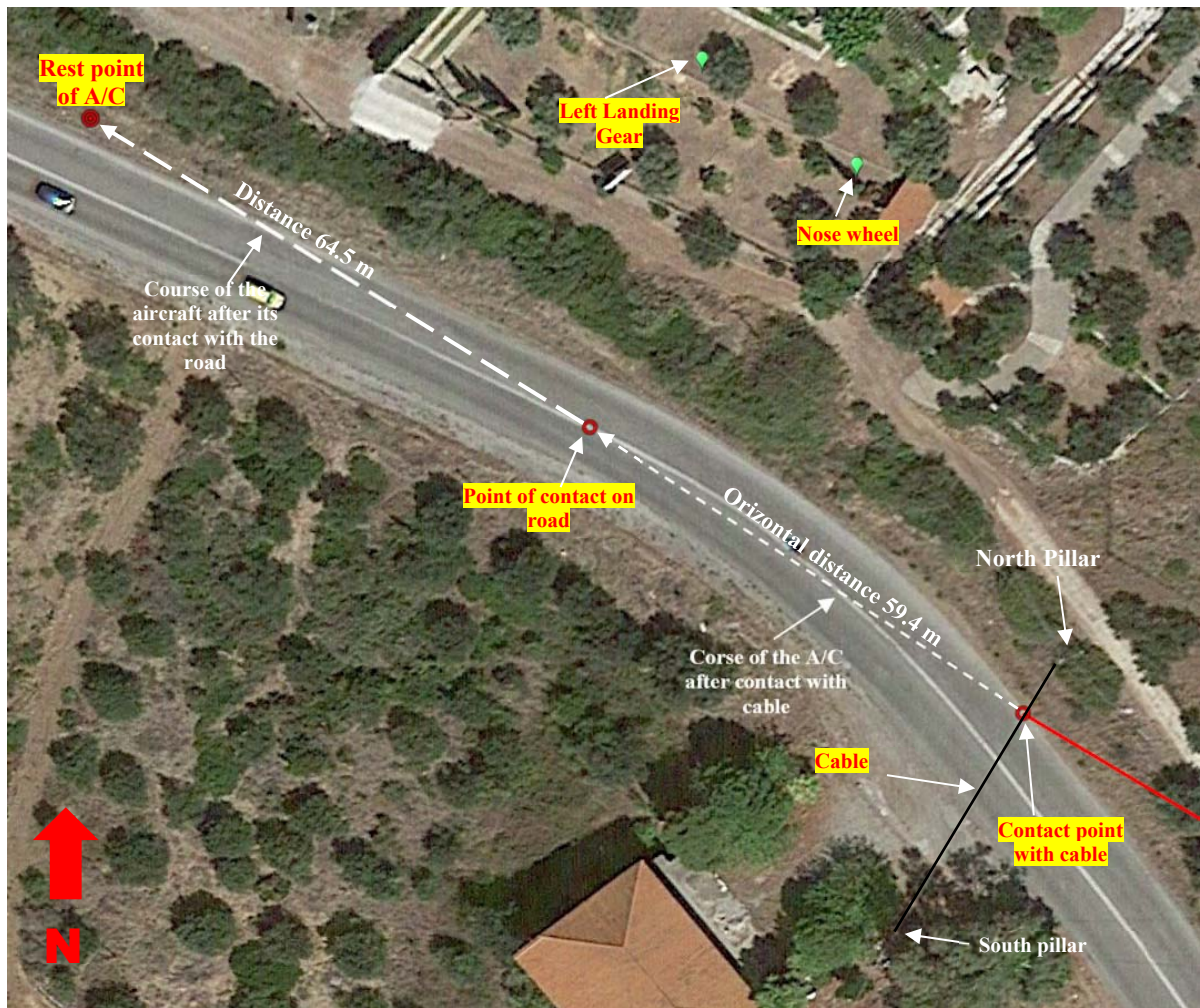
Fig. 5: General view of the accident site.
