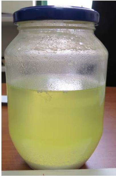
Photo 43: The 6.6% acrylic resin solution immediately after its preparation.
