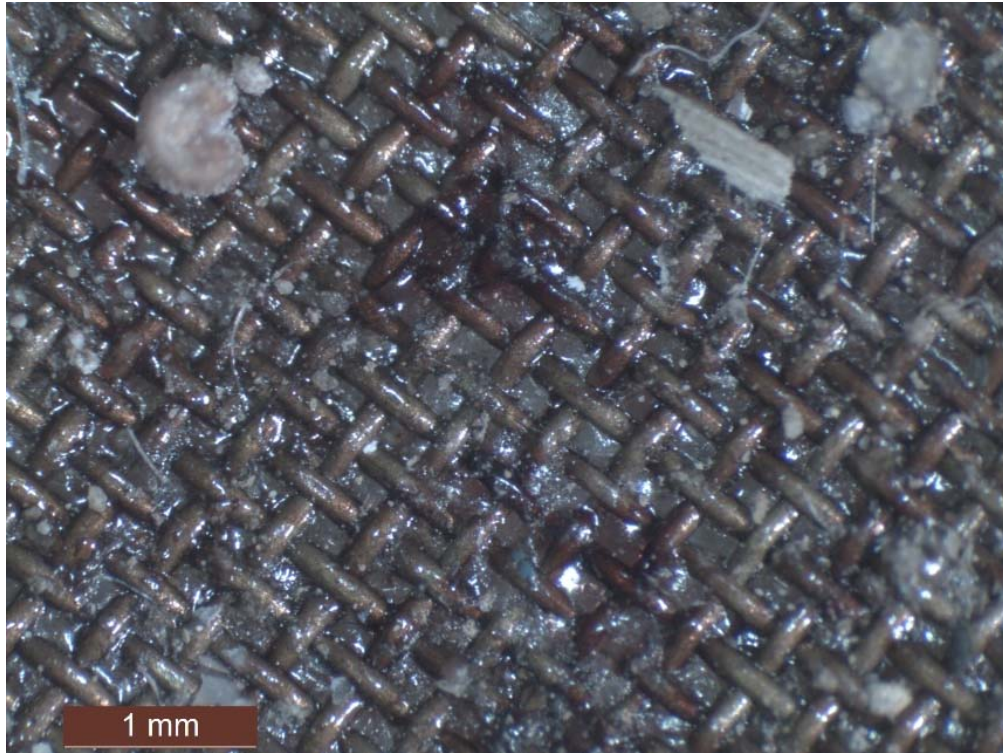
Photo 30: View of fuel filter with glassy material
