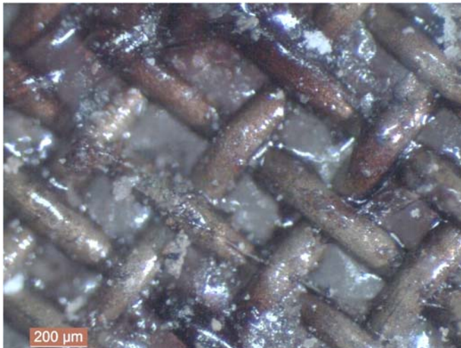
Photo 31: View of the glass material at a larger magnification.
