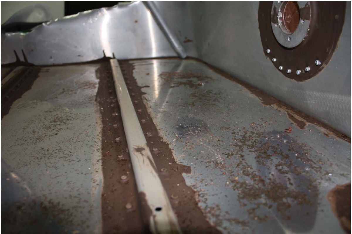
Photo 34: Right hand fuel tank after being opened
