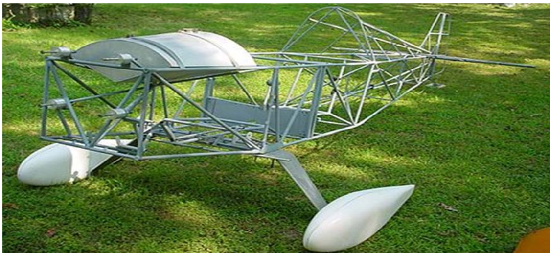
Photo 4: SONERAI II to depict steel tubes aircraft fuselage construction.
