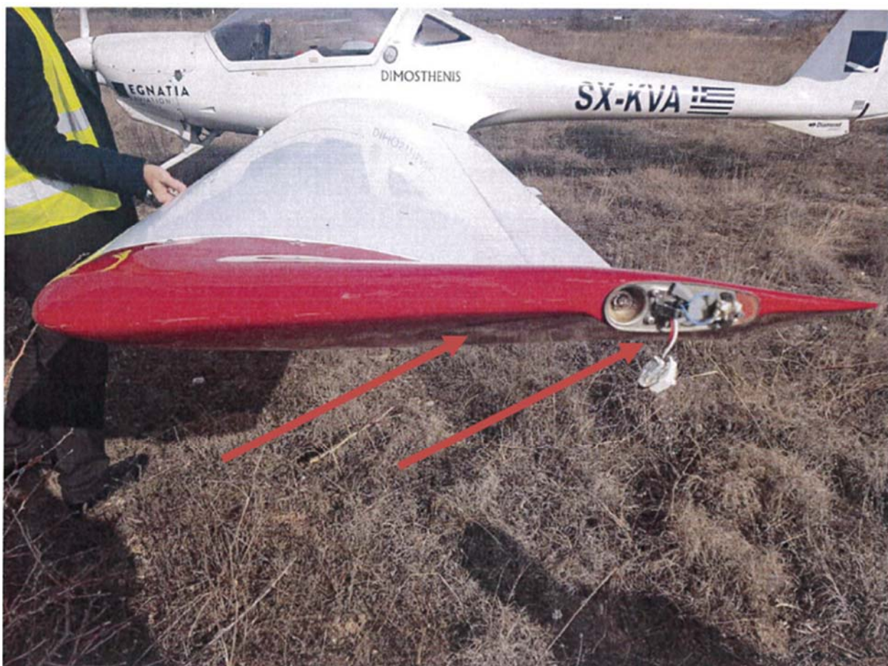
Photo 4: Left wing tip damages.
