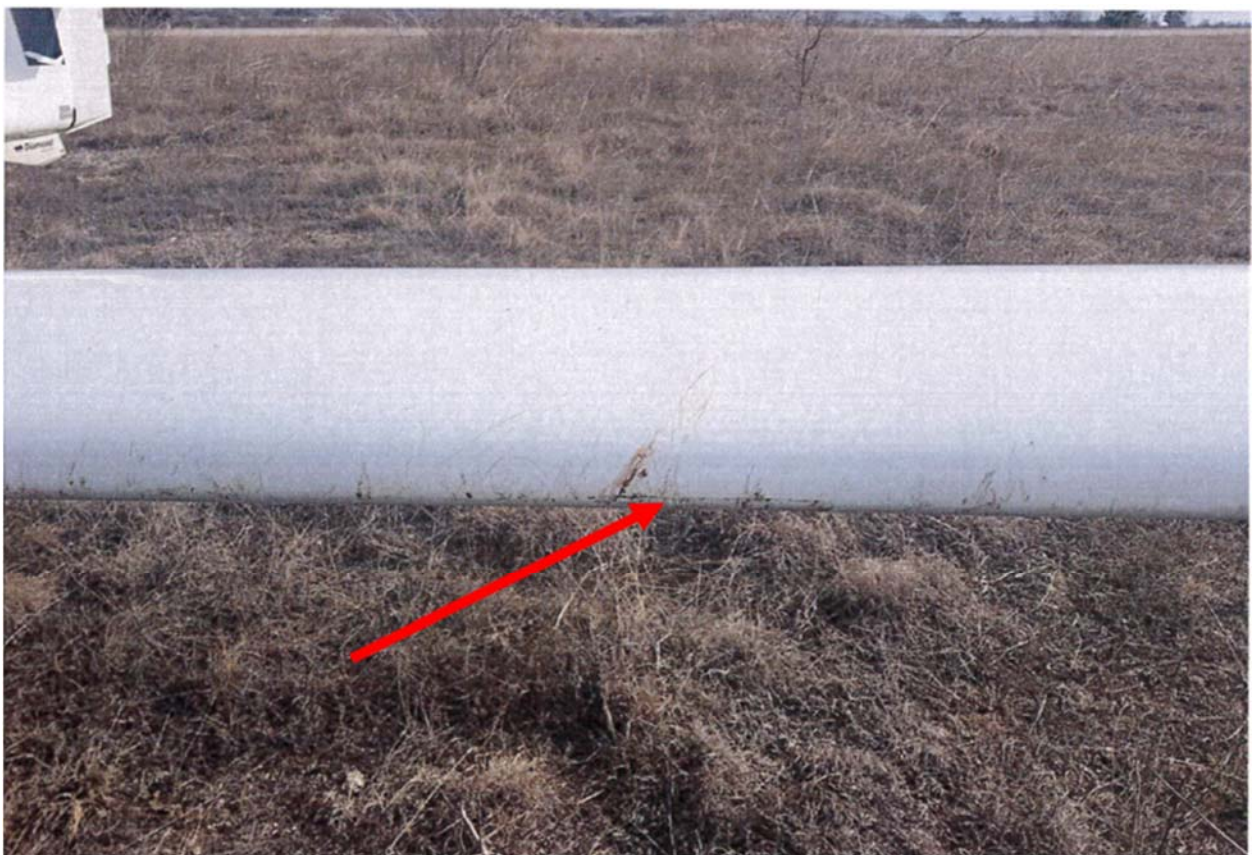
Photo 2: Left wing leading edge with the 22 mm crack.
