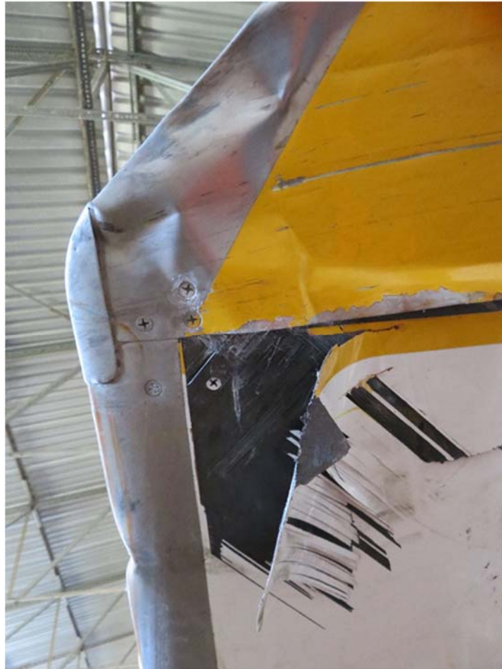
Photo 32: The tip of the white blade with the existing deformations.
