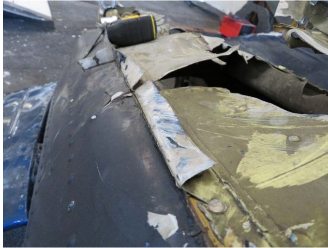
Photo 9: Deformations in the area of the Shaft of rotation of the Tail Rotor. The photo has a forward direction.
