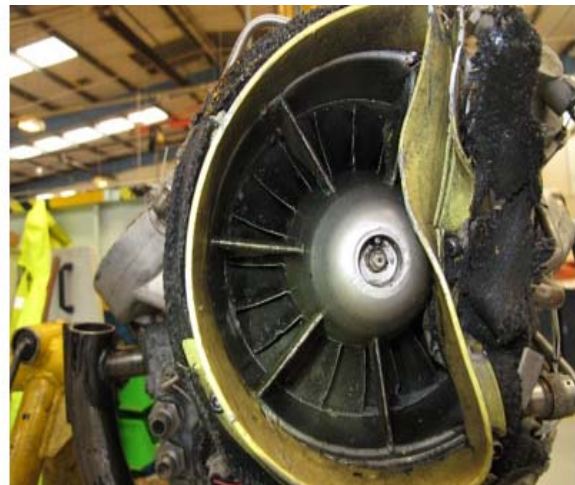
Photo 14: The intake of the right engine compressor with the deformation of its front support part.
