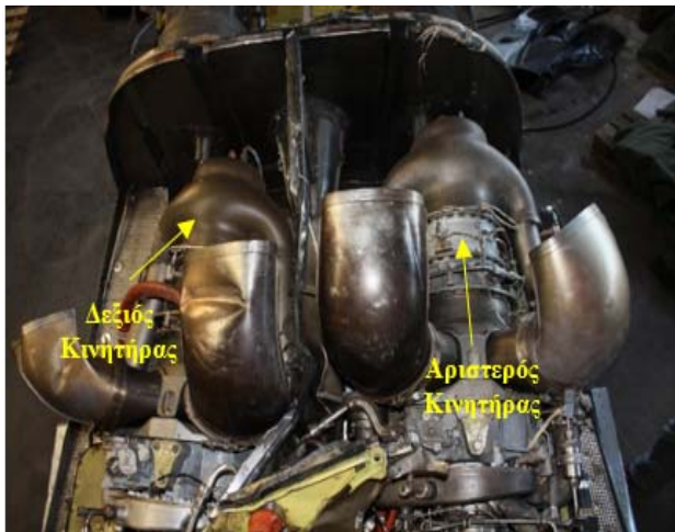
Photo 13: The axial displacement of the right motor to the left .
