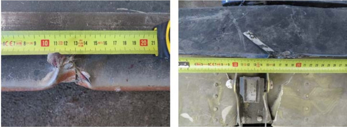
Photo 30: The 5 cm length impact on the edge of the white blade and of the same dimension at the base of the bearing support of tail rotor shaft.
