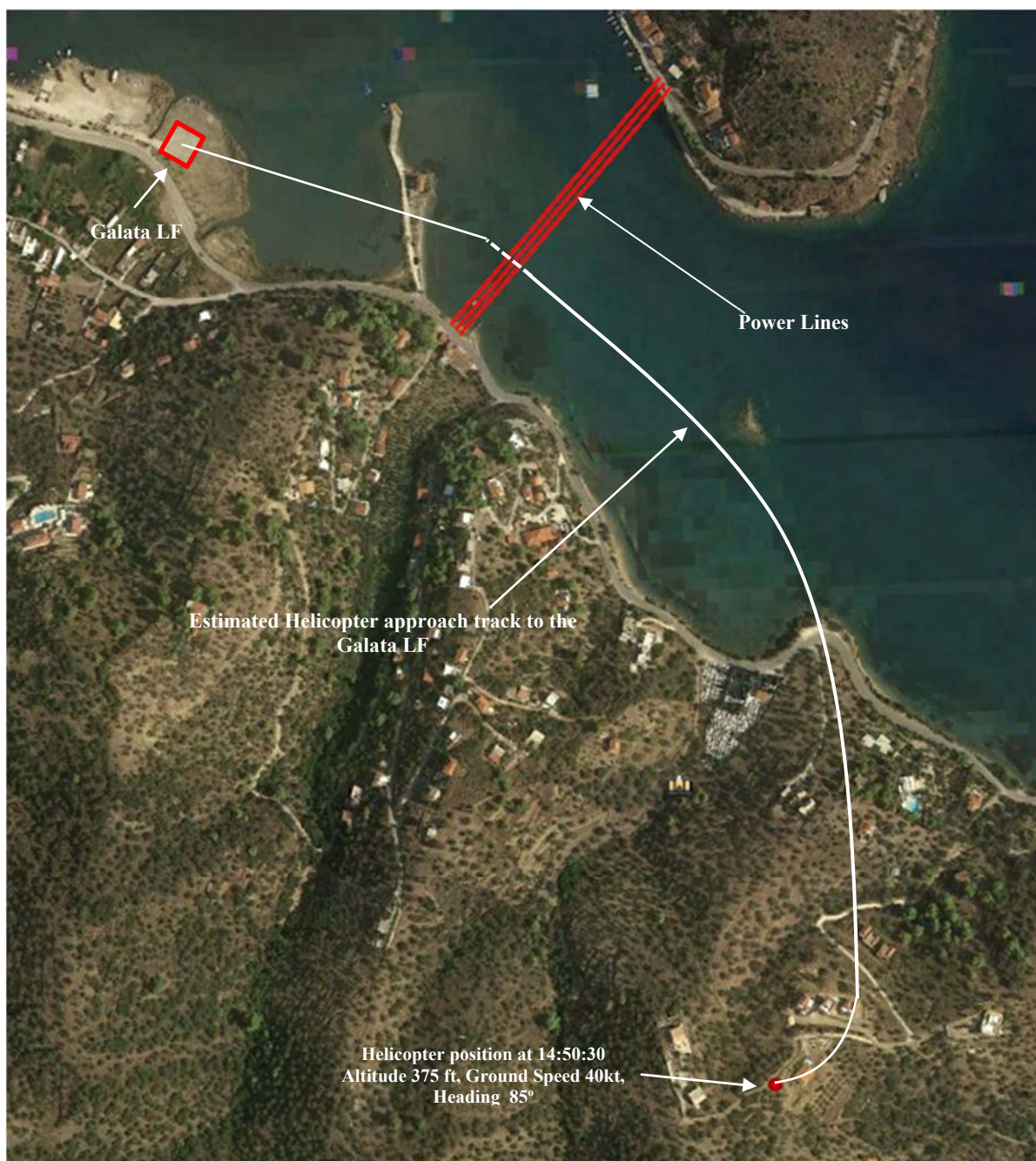
Fig. 7: Estimated Helicopter track during approach for landing at Galata LF. The dotted line represents the flight under the Power Cables.
