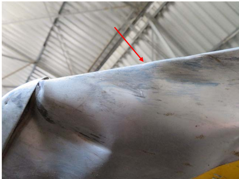
Photo 33: The tip of the white blade with color imprints from the impact on the tail section (red arrow).
