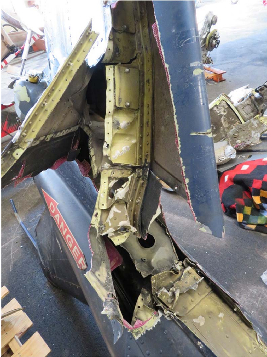
Photo 29: Deformations of the vertical fixed tail section.
