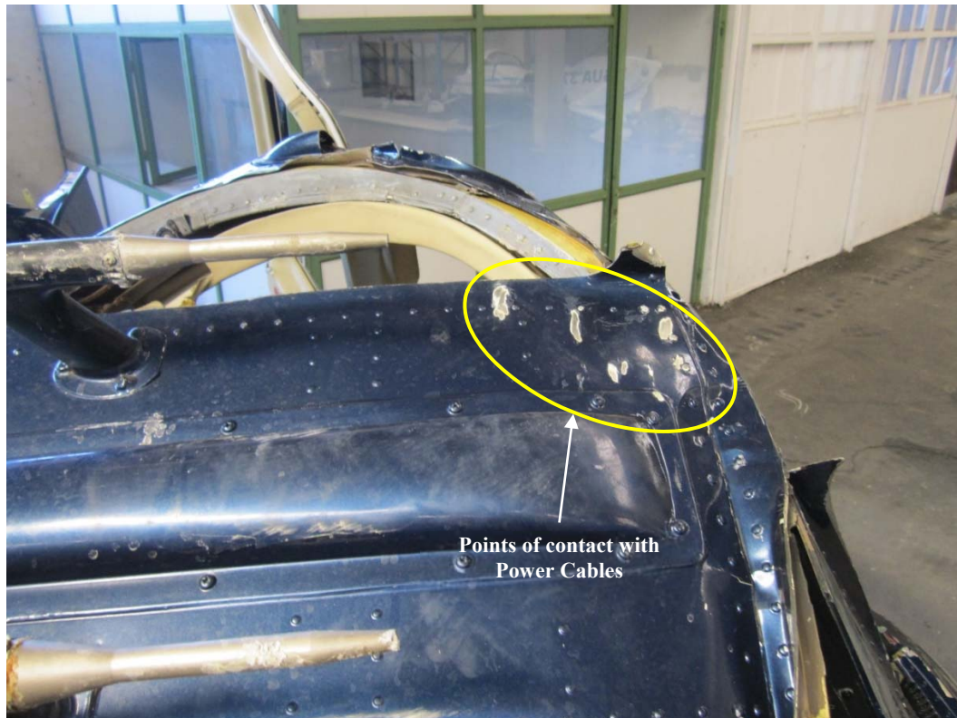
Photo 22: The points of contact of the Helicopter cockpit upper part with the Power Cables.
