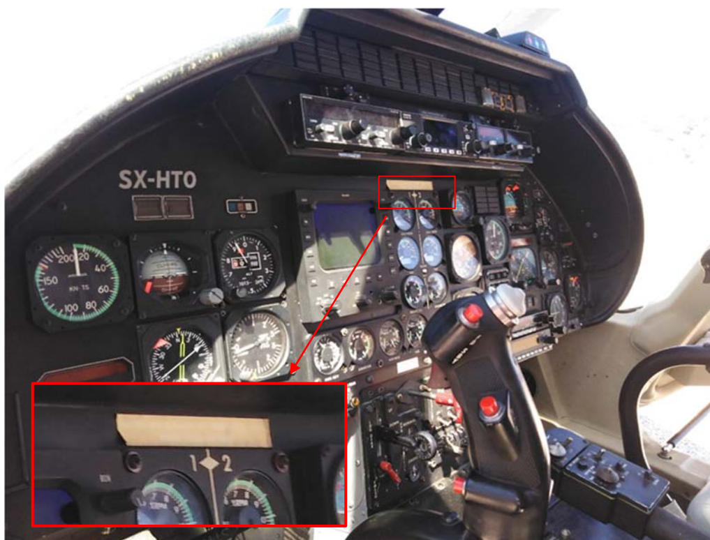
Photo 42: The numbering of the engines in the instrument panel.
