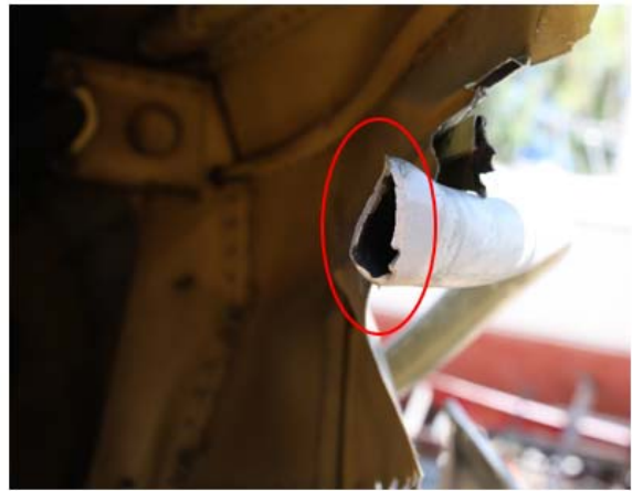
Photo 45: The breaking point of the tail rotor shaft.
