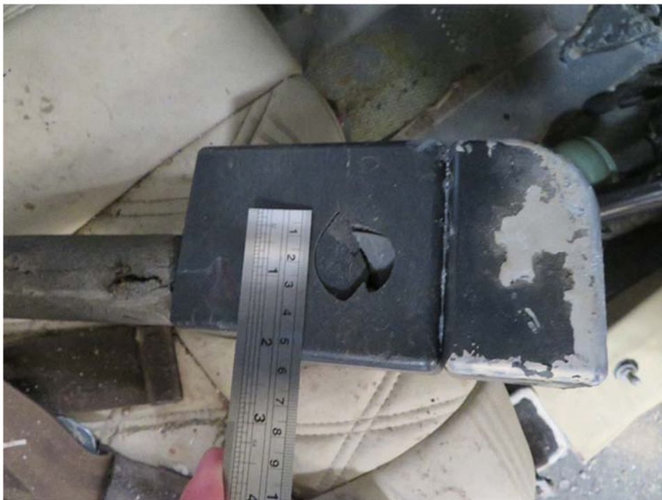
Photo 40: Collective control lever perforation.
