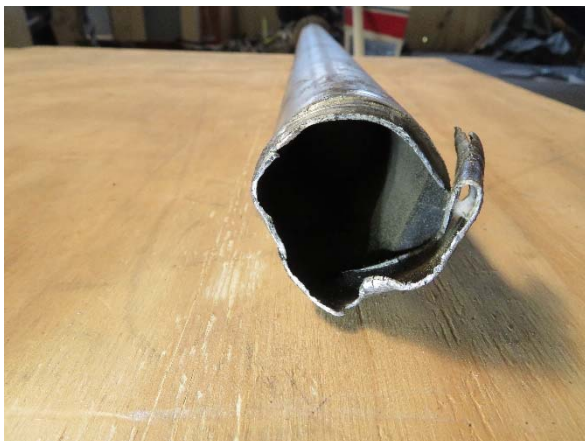
Φωτ. 1: The tail shaft's forward section fracture point
