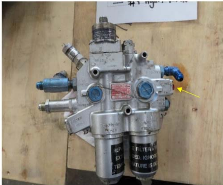
Φωτ. 10: The No1 hydraulic filter assembly with the indicative extended (yellow arrow) of the return filter.
