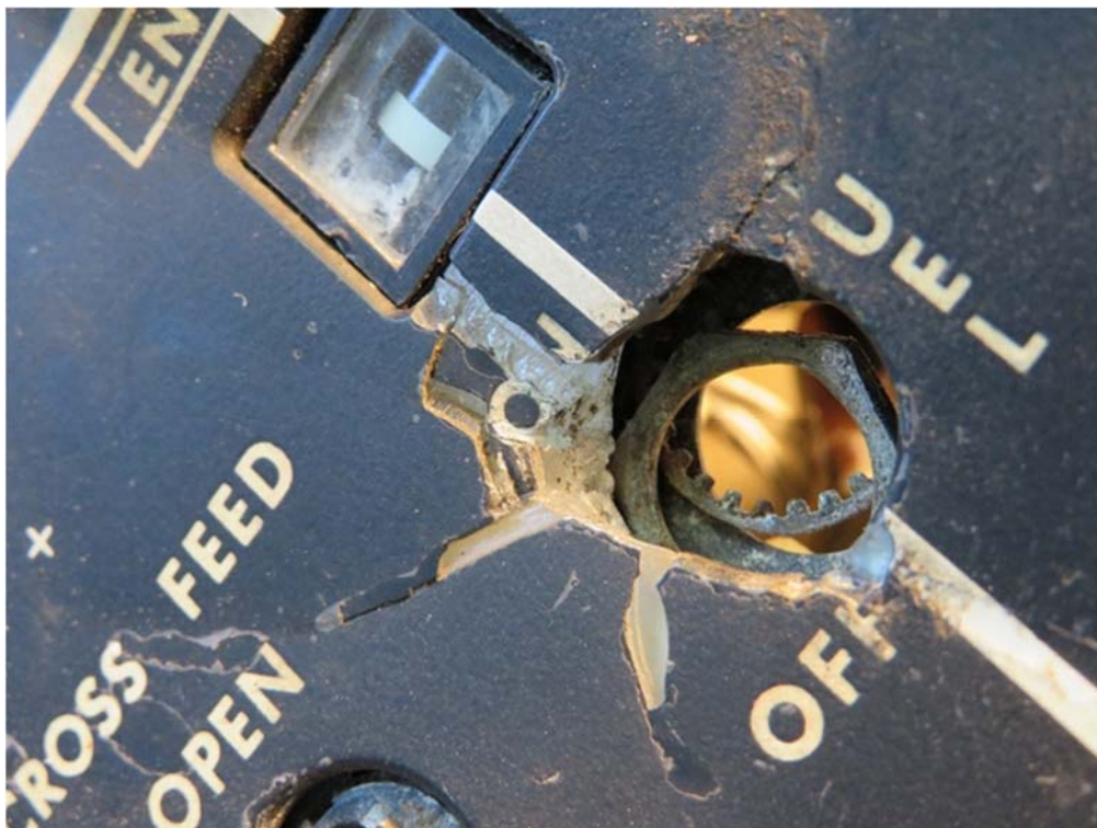
Photo 35: The control panel after removing the switch.
