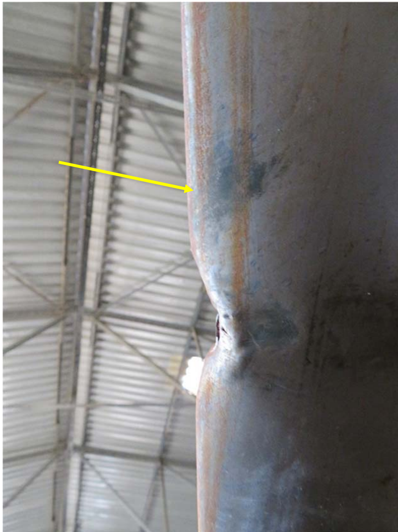
Photo 31: Imprint on the blade from the Helicopter color with the tail section (yellow arrow).
