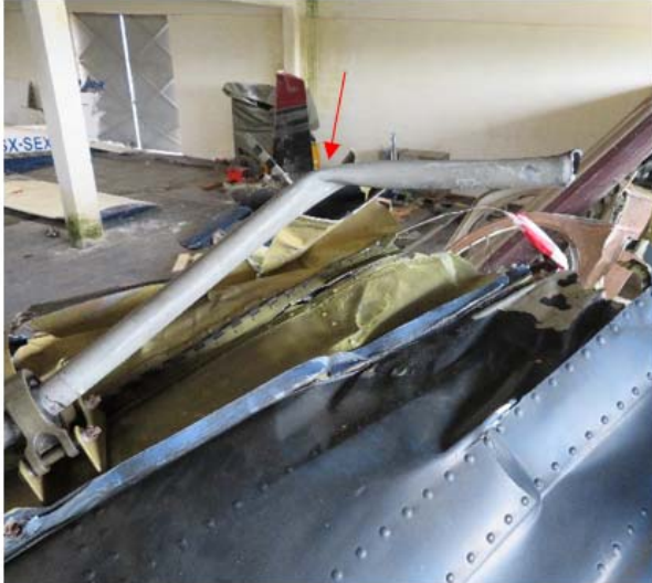
Photo 44: The twist of the rotation axis of the tail rotor (red arrow).
