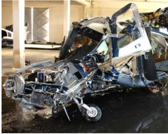
Photo 6: Upward deformation of the forward fuselage section
