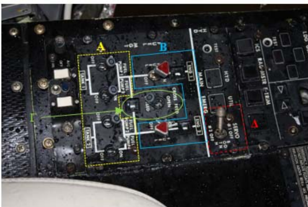
Photo 48: Cockpit view showing the positions of the fuel system switches and the hydraulic systems.
