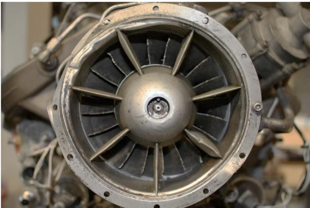
Photo 12: Left Engine Compressor Inlet and its Front Support.
