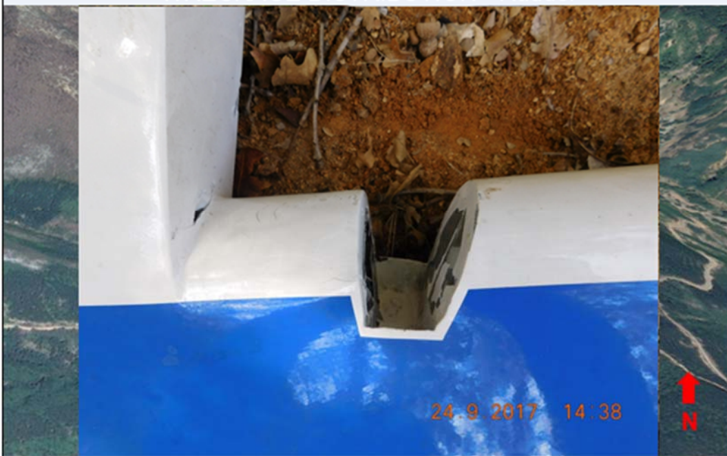
WRECKAGE DISTRIBUTION - Rudder
