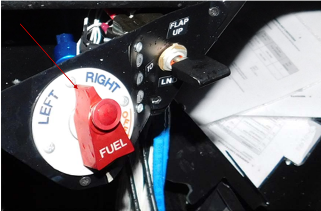
Photo 6: Fuel Tank Selector Switch.
