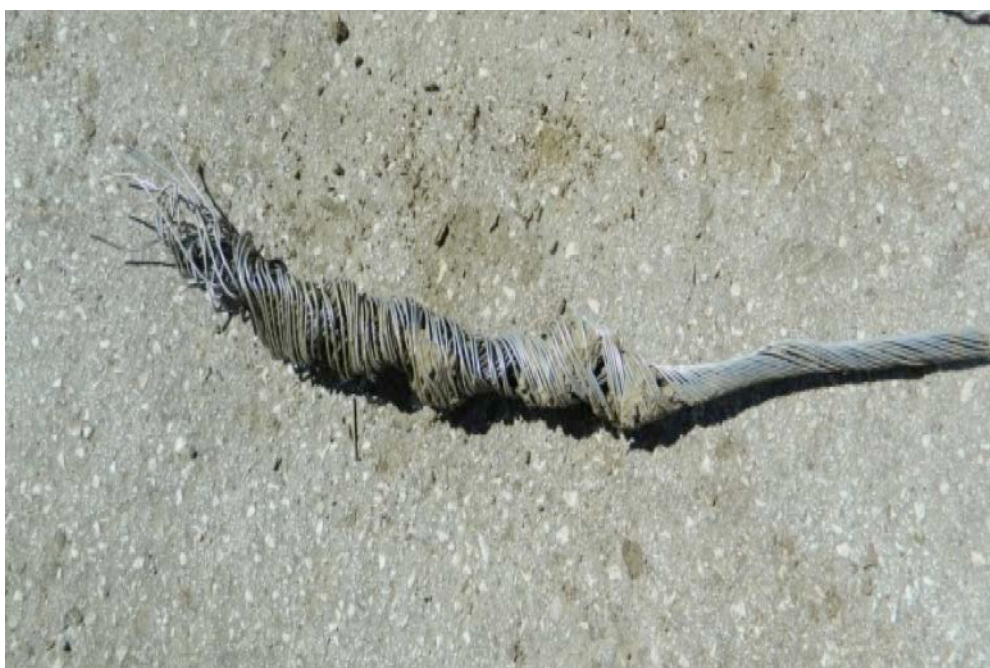
Photo 7. Severed cable end
