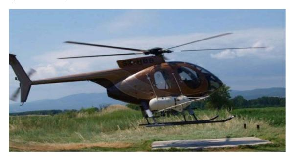
Photo 4: The helicopter fitted with the spraying apparatus
