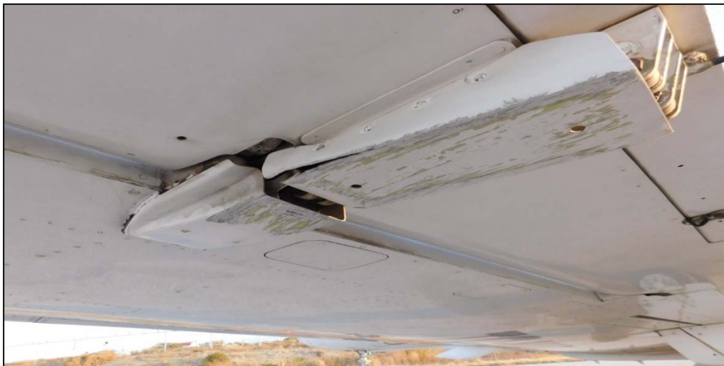
Photo 3: Damage of the left aileron drive cover on the lower part of the left wing.
