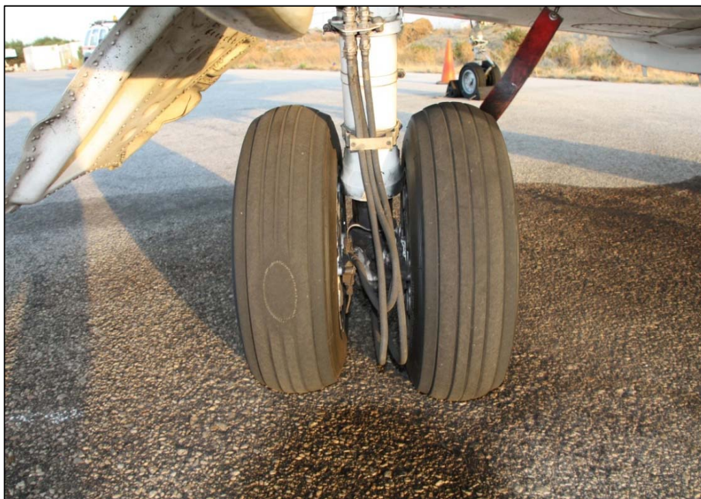
Photo 4: Wear to the outer tire of the left main landing gear.
