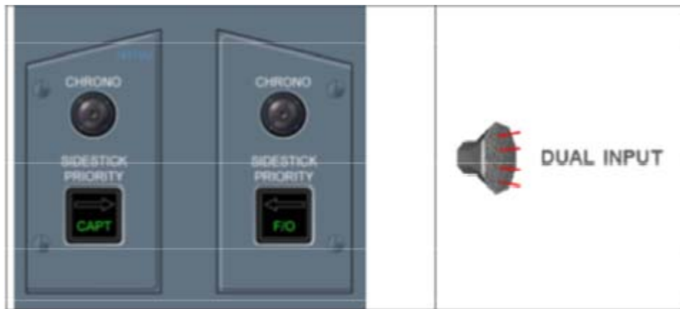
Fig. 19: both Pilots are moving their sidestick without anyone having priority with the activation of the aural sound “DUAL INPUT”
