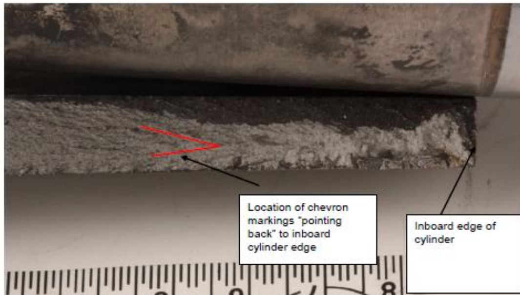
Figure 9: Showing the detail of fracture surface 'A2'.
