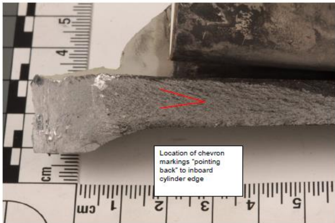
Figure 10: Showing the detail of fracture surface 'A2'.
